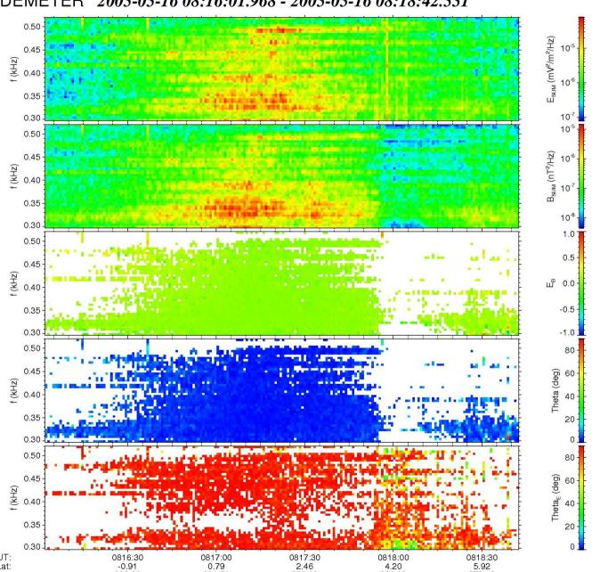
PSD of electric field fluctuations
