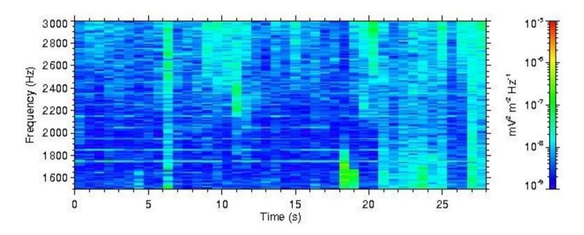
~100 events in VLF range, Burst mode (waveform of 1 electric & 1 magnetic comp.)
