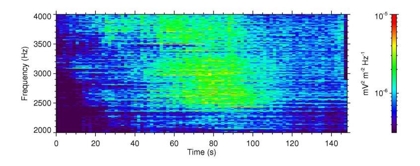
>500 events in VLF range, Survey mode (spectrum of 1 electric & 1 magnetic field component)
