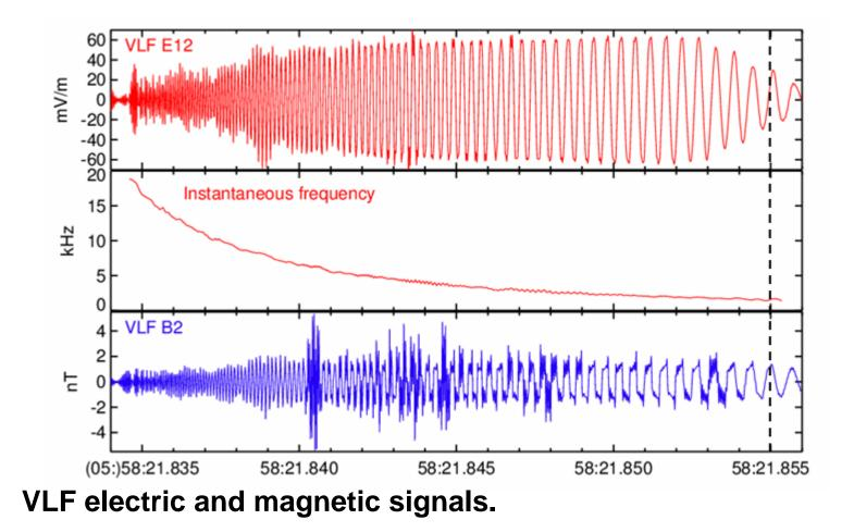
Instantaneouos frequency from the time derivative of the instantaneous phase of an analytic signal (using the discrete Hilbert transform)
