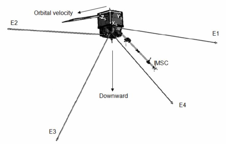
ICE electric antennas E1, E2, E3, and E4 : 30-mm spheres on 4.5-m booms. Three-axial search coil magnetometer IMSC: on a 2.5-m boom. The spacecraft coordinate system  $X_s$ ,  $Y_s$ ,  $Z_s$ .
